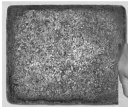
Oil Stained Pavement Stone
